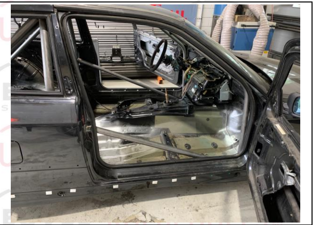
PHOTO 11 ANTI-INTRUSION DOORBAR – CO-DRIVER
