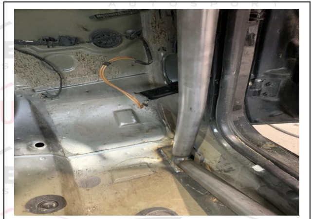
PHOTO 6 FRONT ROLLBAR TO FLOOR ATTACHMENT
