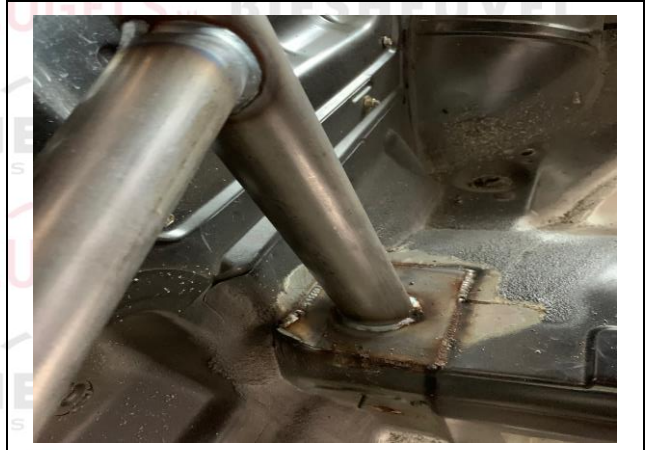
PHOTO 4 MAIN ROLLBAR TO FLOOR ATTACHMENT
