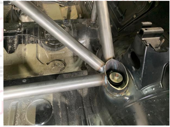
PHOTO 13 SHOULDER HARNESS ATTACHMENT - CO DRIVER
