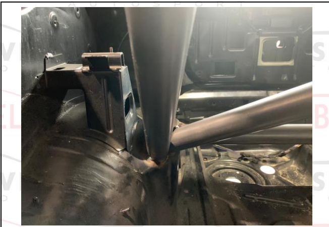
PHOTO 5 REAR BACKSTAY TO BODYSHELL ATTACHMENT
