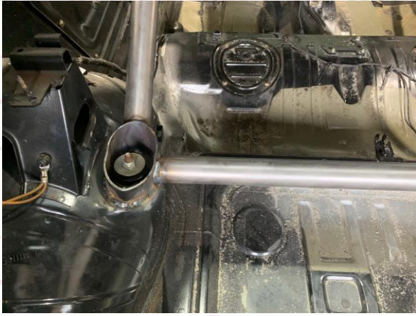
PHOTO 12 SHOULDER HARNESS ATTACHMENT - DRIVER
